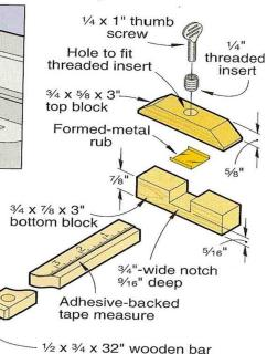
measuring bar in front of the sawblade and extend it out until it touches the fence. Now, tighten the thumbscrew. Place the gauge in the miter slot at the back of the table, check the measurement to the fence, and repeat the procedure on the front of the table. Adjust the fence until it reads exactly the same distance at both the front and the back of the table.
